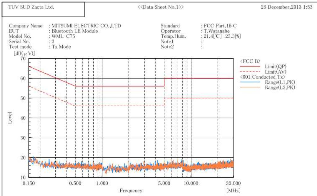
Note: No emissions were observed during Conducted Emission testing.
