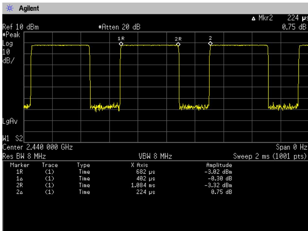
$$\text{Duty Cycle} = T_{\text{on}} / (T_{\text{on}} + T_{\text{off}}) = 402[\mu\text{s}] / (402[\mu\text{s}] + 224[\mu\text{s}]) = 64.22[\%]$$
