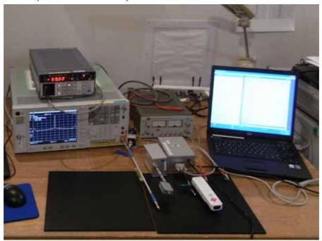
Transmitter Radiated Spurious Emissions (RF Radiated test)
