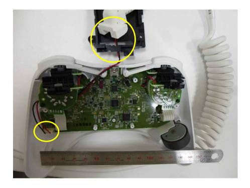
Same PCB used as "model: WUP-005" only power is connected directly to cable instead of rechargeable battery and battery case.
