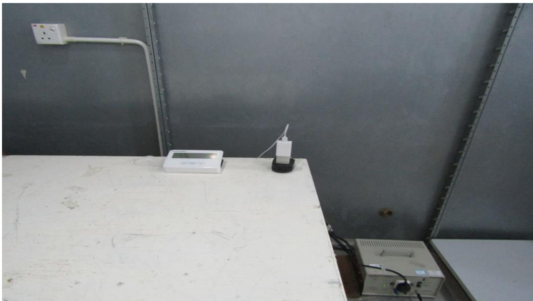
Measurement of Conducted Emission Test Set Up
