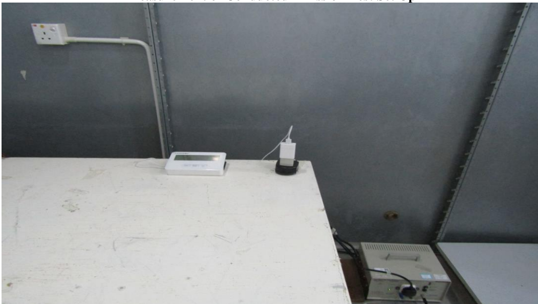
Measurement of Conducted Emission Test Set Up
