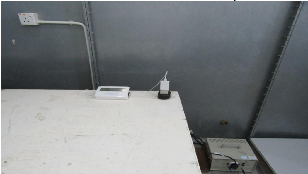
Measurement of Conducted Emission Test Set Up
