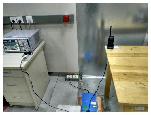
RADIATED EMISSION TEST SETUP
