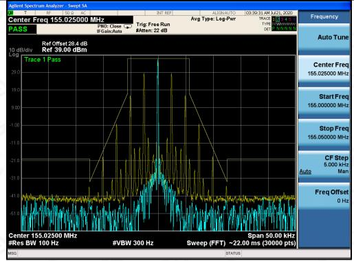
The Worst Emission Mask for (173.975 MHz) of 12.5 KHz channel Separation (5W)
