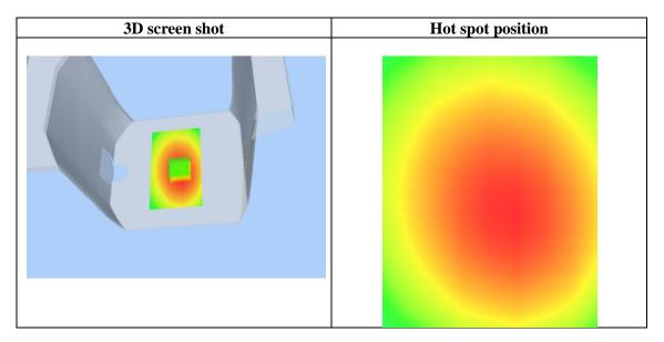
Test Laboratory: AGC Lab CW300High- face up 2.5cm **DUT: Two-way Radio; Type: TH-UVF9** Communication System: CW; Communication System Band: CW173.975 MHz; Duty Cycle: 1:1; Conv.F=4.58 Frequency:173.975 MHz; Medium parameters used: f = 300MHz;  $\sigma$  = 0.89mho/m;  $\epsilon$ r = 44.96; $\rho$  = 1000 kg/m<sup>3</sup>; Phantom Type: Elliptical Phantom Ambient temperature (°C): 21.5, Liquid temperature(°C): 21.0
