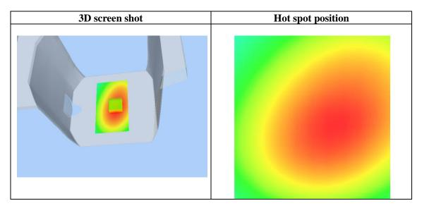
Test Laboratory: AGC Lab CW450 Low- Face up 2.5 cm separation DUT: Two-way Radio; Type: TH-UVF9 Communication System: CW; Communication System Band: CW 407.625 MHz; Duty Cycle: 1:1; Conv.F=4.75 Frequency: 407.625 MHz; Medium parameters used: f = 450 MHz;  $\sigma$  = 0.91 mho/m;  $\epsilon$ r = 43.56;  $\rho = 1000 \text{ kg/m}^3$ ; Phantom Type: Elliptical Phantom
