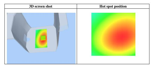
Test Laboratory: AGC Lab CW300High- bottom -touch DUT: Two-way Radio; Type: TH-UVF9 Communication System: CW; Communication System Band: CW 173.975 MHz; Duty Cycle: 1:1; Conv.F=4.58 Frequency: 173.975 MHz; Medium parameters used: f = 300MHz;  $\sigma = 0.91$ mho/m;  $\epsilon r = 57.72$ ;  $\rho = 1000 \text{ kg/m}^3$ ; Phantom Type: Elliptical Phantom Ambient temperature (°C): 21.5, Liquid temperature(°C): 21.0
