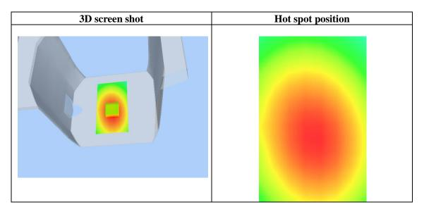
Test Laboratory: AGC Lab CW450 Middle- Face up 2.5 cm separation DUT: Two-way Radio; Type: TH-UVF9
