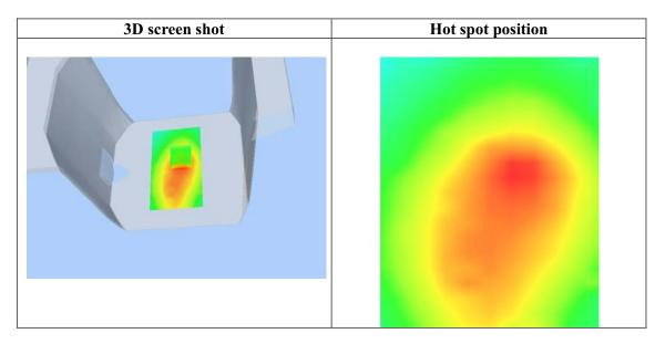
Test Laboratory: AGC Lab CW300High- face up 2.5cm **DUT: Two-way Radio; Type: TH-UV3R** Communication System: CW; Communication System Band: CW173.975 MHz; Duty Cycle: 1:1; Conv.F=4.58 Frequency:173.975 MHz; Medium parameters used: f = 300MHz;  $\sigma$  = 0.89mho/m;  $\epsilon$ r = 44.96; $\rho$  = 1000 kg/m<sup>3</sup>; Phantom Type: Elliptical Phantom Ambient temperature (°C): 21.5, Liquid temperature(°C): 21.0
