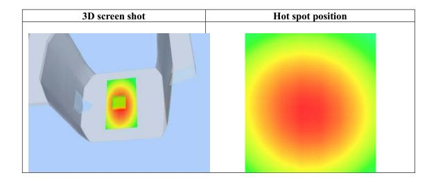
Test Laboratory: AGC Lab CW450 Middle- Face up 2.5 cm separation DUT: Two-way Radio; Type: TH-UV3R
