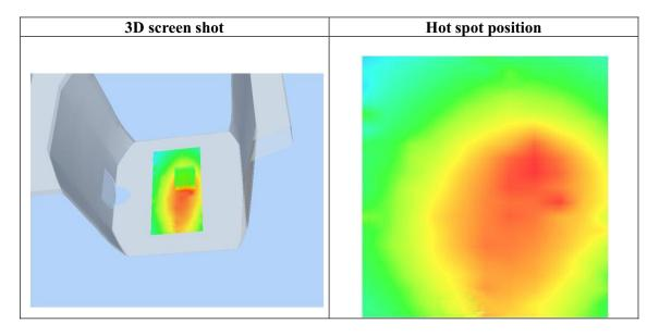
Test Laboratory: AGC Lab CW300Low-bottom- touch **DUT: Two-way Radio; Type: TH-UV3R**  Test date: Mar.25, 2013
