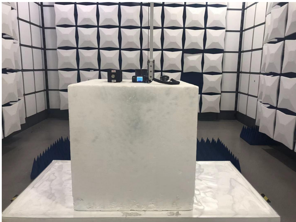
RADIATED EMISSION ABOVE 1G TEST SETUP
