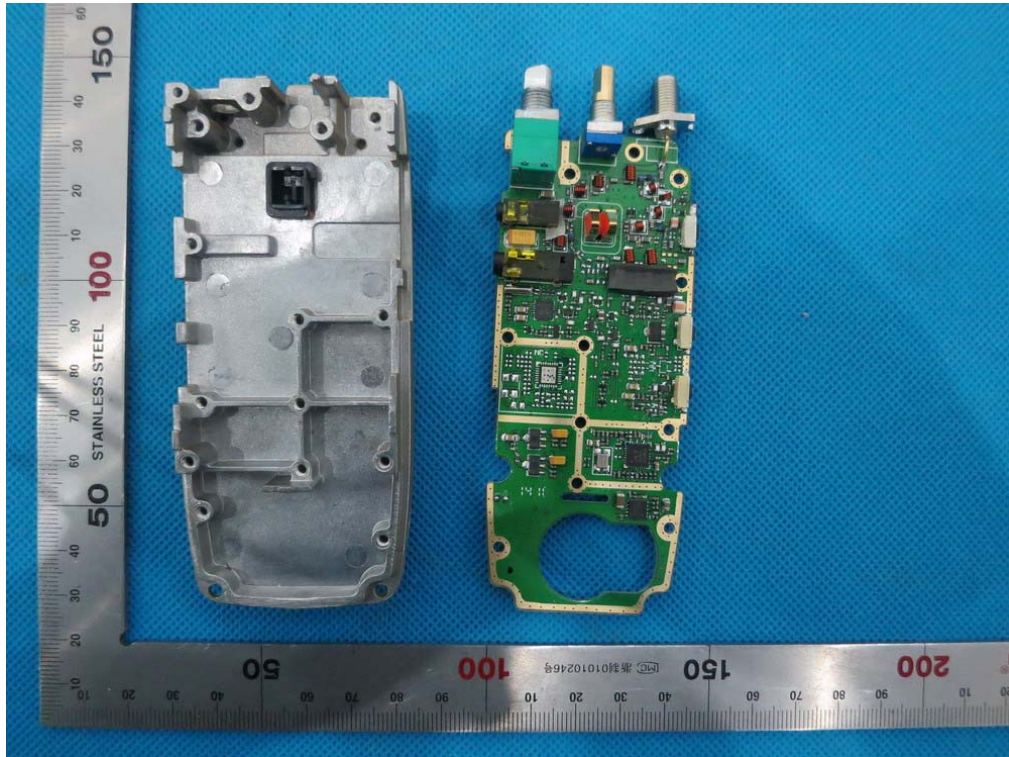
INTERNAL VIEW OF EUT-5
