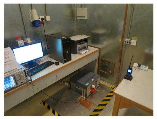
CONDUCTED EMISSION TEST SETUP
