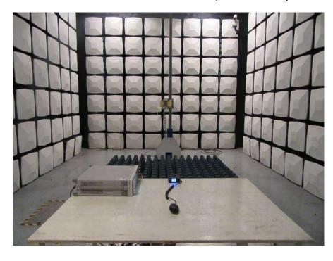
Radiated Emission - Rear View (Above 1 GHz)
