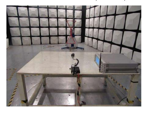
Radiated Emission - Front View (Above 1 GHz)
