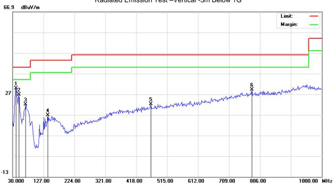
Radiated Emission Test --Vertical -3m Below 1G
