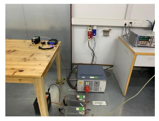
RADIATED EMISSION TEST SETUP-BELOW 1GHZ
