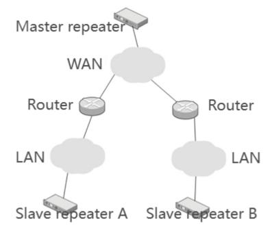
As shown in the above photo, the Slave A and the Slave B are distributed in different LANs, and the two LANs are in different networks. If it is necessary to make port mapping, the Slave must have a static internal network IP address, and make port mapping through a router, so as to realize the connection with the master repeater and other Slaves. For the port mapping setting methods, please refer to the use instructions of chosen routers.
