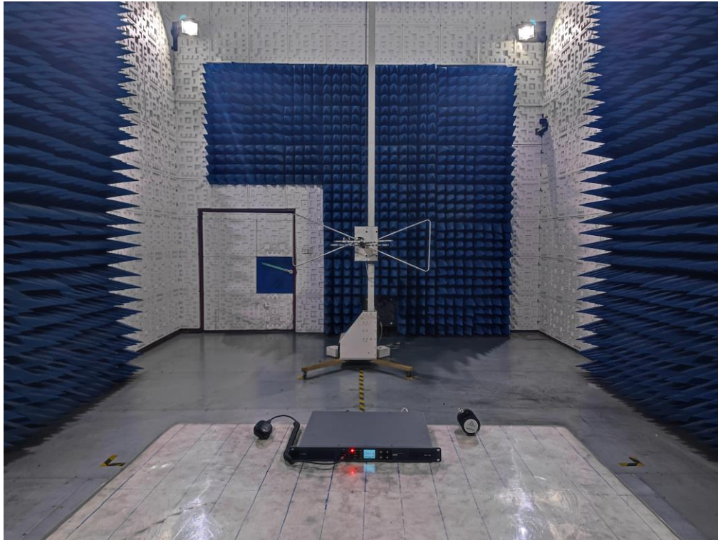
RADIATED EMISSION TEST SETUP ABOVE 1GHz
