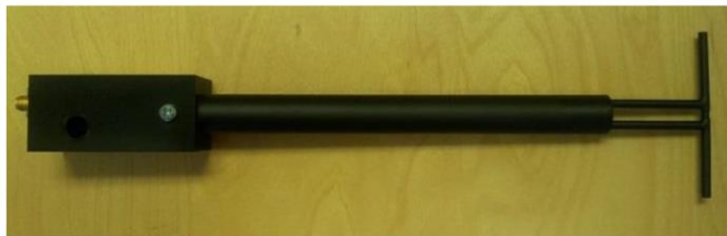
Figure 1 – MVG COMOSAR Validation Dipole
