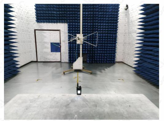
APPENDIX E PHOTOGRAPHS OF TEST SETUP RADIATED SPURIOUS EMISSION
