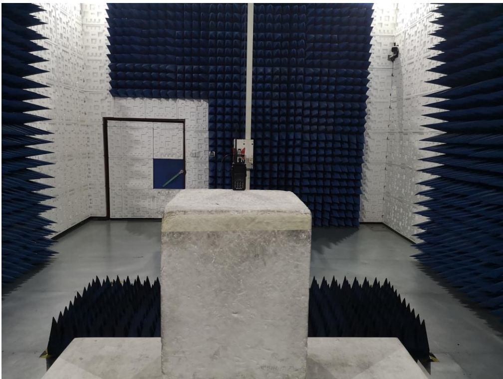
RADIATED EMISSION ABOVE 1G TEST SETUP
