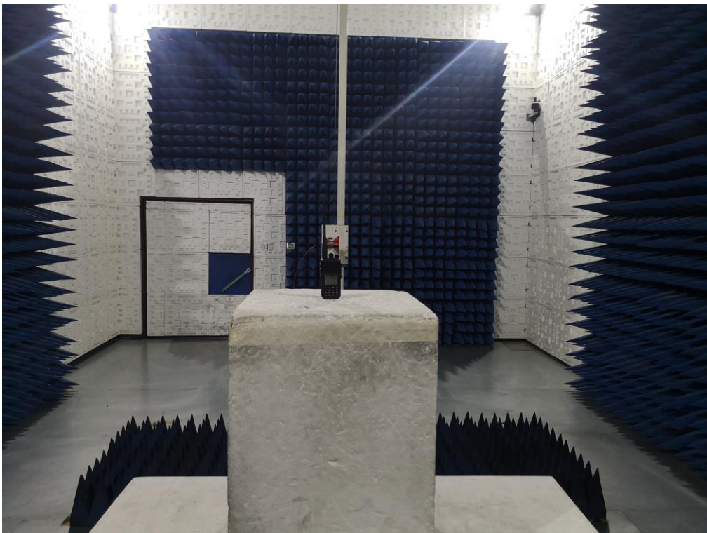
RADIATED EMISSION ABOVE 1G TEST SETUP
