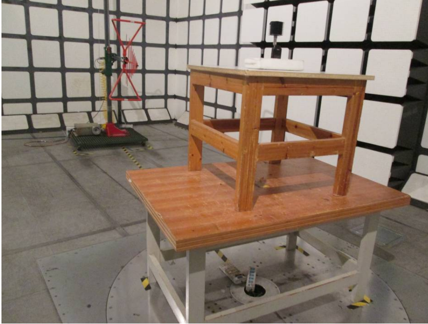
Transmitting Radiated Emissions View (Below 1 GHz)
