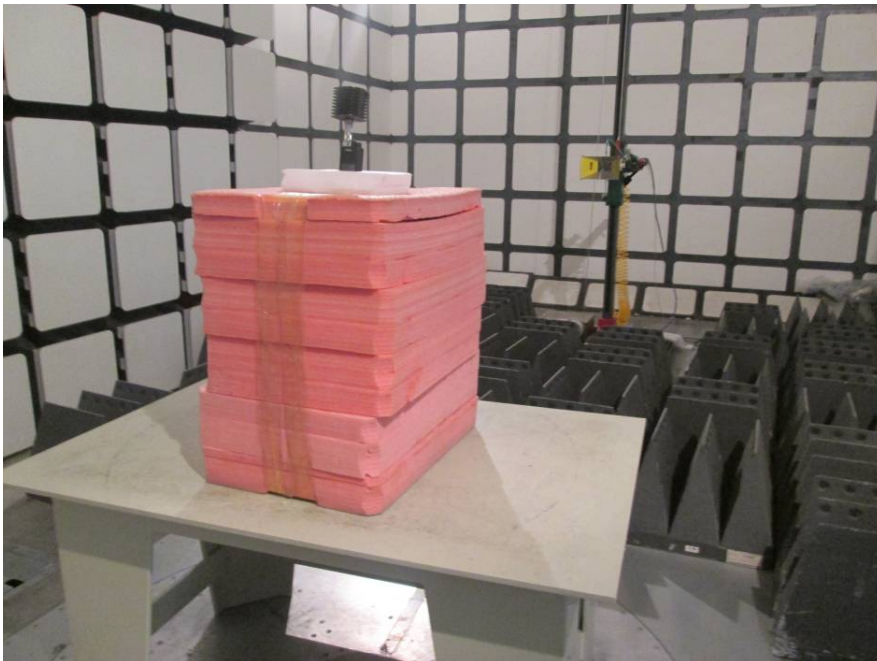
Transmitting Radiated Emissions View (Above 1 GHz)
