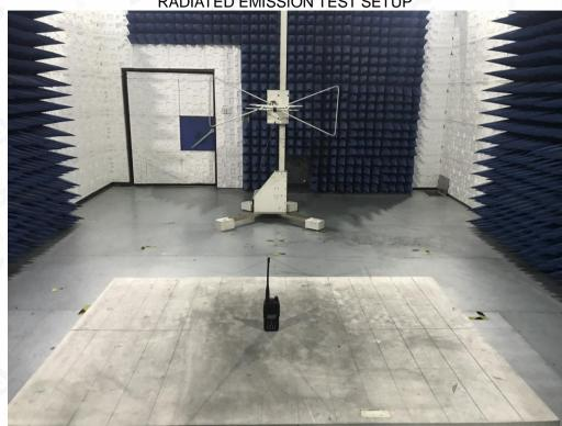
RADIATED EMISSION ABOVE 1G TEST SETUP
