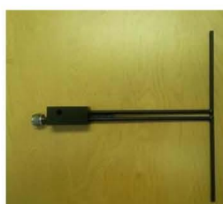
Figure 1 – MVG COMOSAR Validation Dipole
