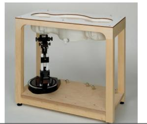
The bottom plate contains three pair of bolts for locking the device holder. The device holder positions are adjusted to the standard measurement positions in the three sections. A white cover is provided to tap the phantom during off-periods to prevent water evaporation and changes in the liquid parameters. On the phantom top, three reference markers are provided to identify the phantom position with respect to the robot.
