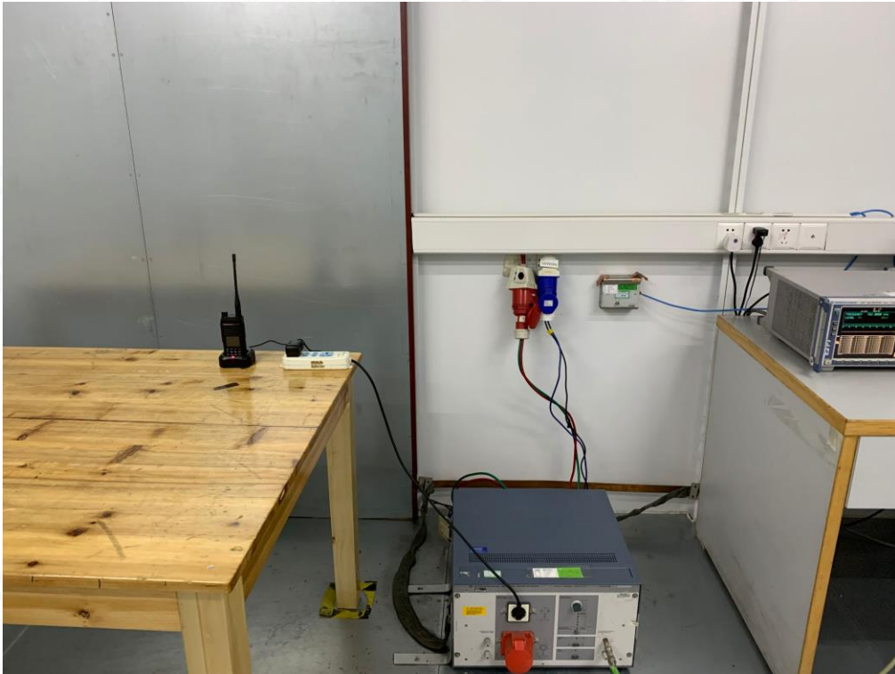
RADIATED EMISSION TEST SETUP-BELOW 1GHZ
