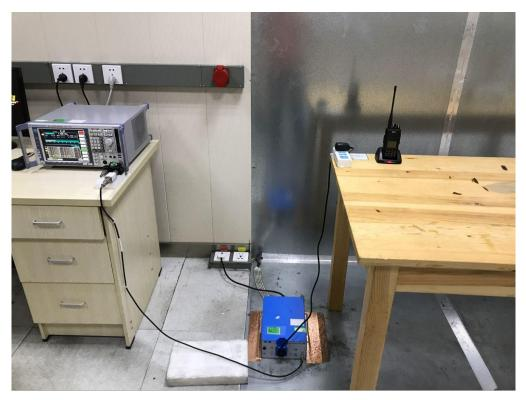
RADIATED EMISSION TEST SETUP
