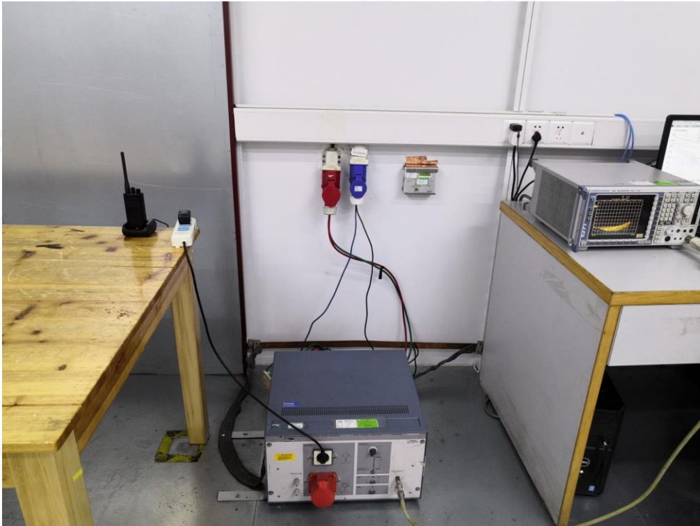
RADIATED EMISSION TEST SETUP-BELOW 1GHZ
