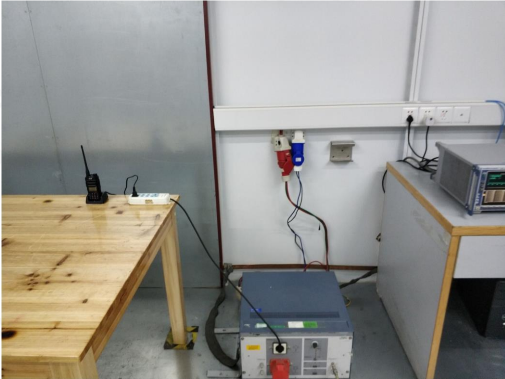
RADIATED EMISSION TEST SETUP-BELOW 1GHZ
