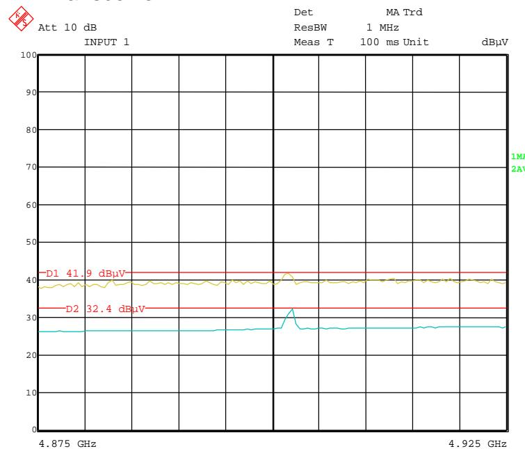
1<sup>st</sup> harmonic emission, normal rated supply voltage 24 VDC, measurement distance 3 m, SR-Transceiver
