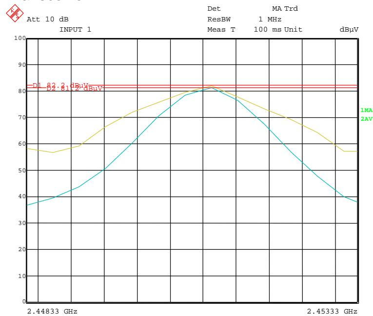
2.45 GHz, normal rated supply voltage 24 VDC, measurement distance 3 m, SR-Transceiver
