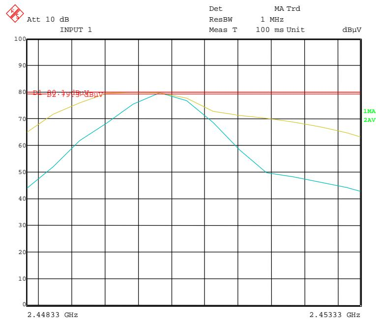
2.45 GHz, extreme voltage supply 27.6 VDC, measurement distance 3 m, LR-Transceiver
