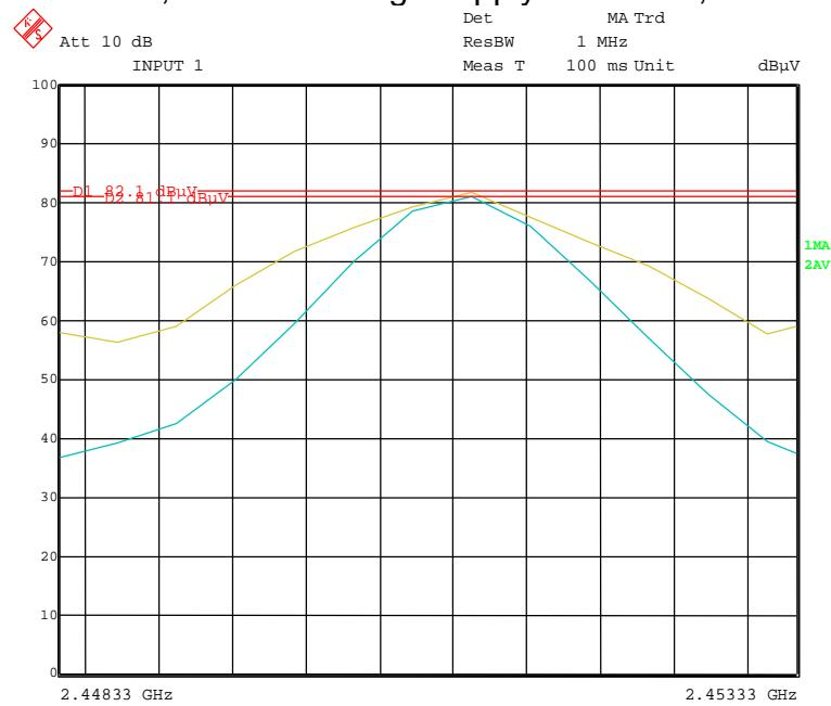
2.45 GHz, extreme voltage supply 20.4 VDC, measurement distance 3 m, SR-Transceiver
