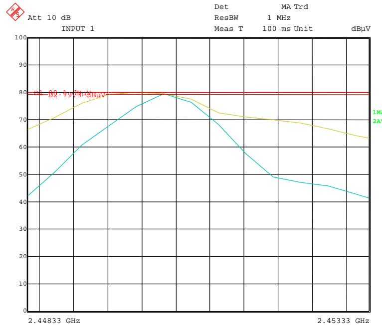
2.45 GHz, extreme voltage supply 20.4 VDC, measurement distance 3 m, LR-Transceiver
