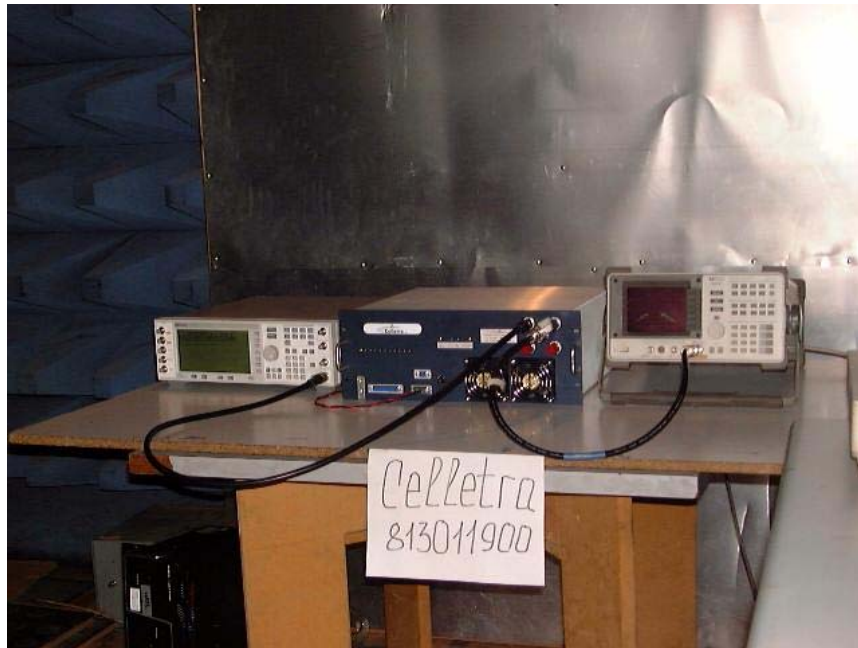
Figure 32. Effective Radiated Power Test Setup
