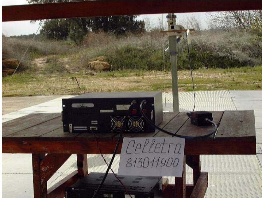
Figure 34. Out of Band Emission (Radiated) Test Setup
