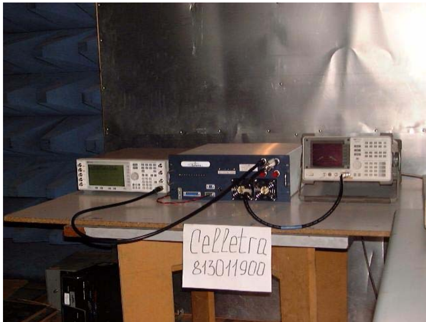
Figure 35. Out of Band Emissions at Antenna Terminals Test Setup
