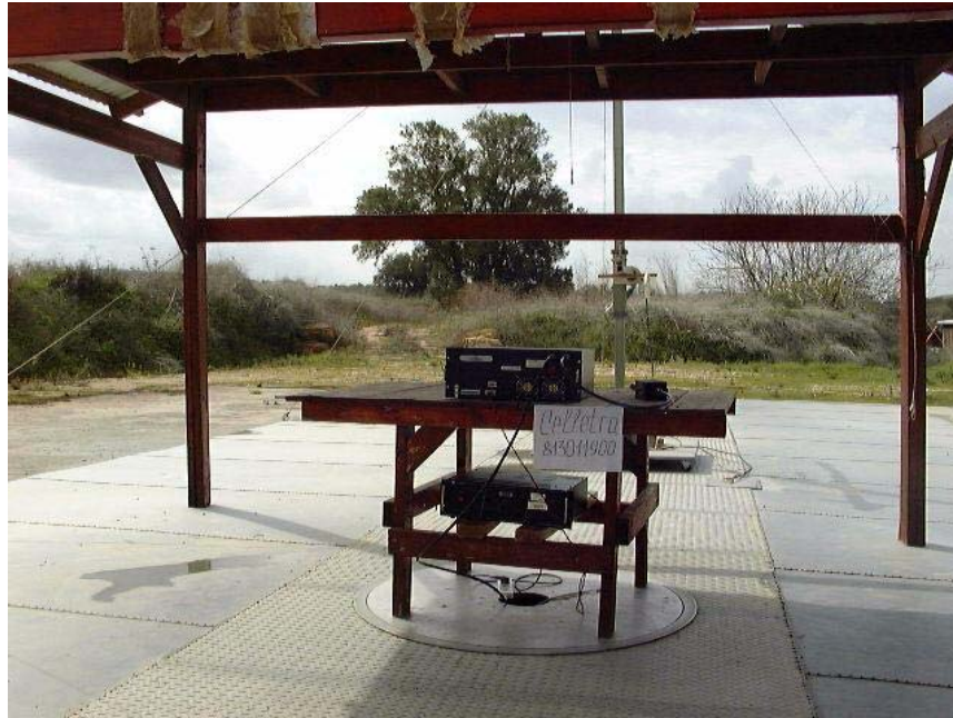
Figure 36. Radiated Emission Part 15 Test Setup
