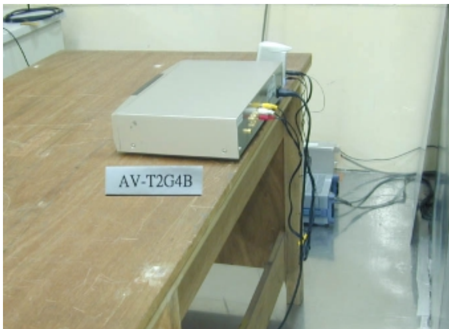
Photo 2: Conducted Emission Test Set-up (rear)
