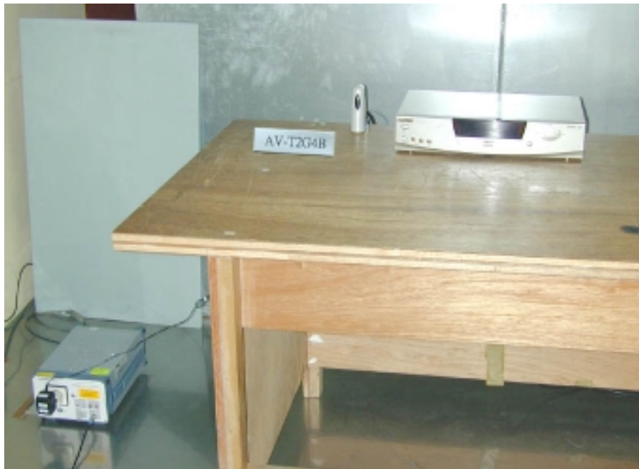
Photo 2: Conducted Emission Test Set-up (rear)
