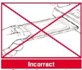
Do not handle or remove the PCS Connection Card by pulling on the antenna.
