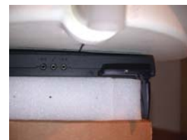
Figure 14.9 Body SAR Test Setup -- Lap Configuration --
