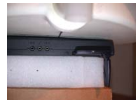
Figure 14.11 Body SAR Test Setup -- Lap Configuration --
