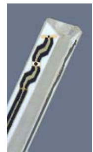
Figure 3.2 Probe Thick-Film Technique
