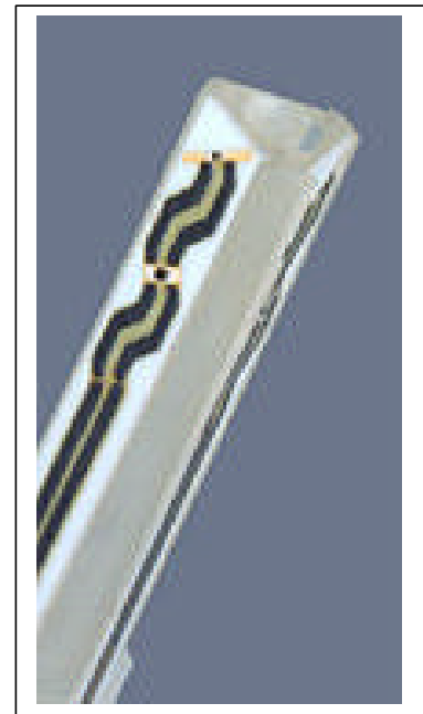
Inside view of ET3DV6 E-field Probe
