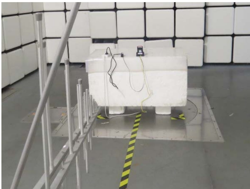
Mode 4(Adapter + EUT +camera on + wifi on)
