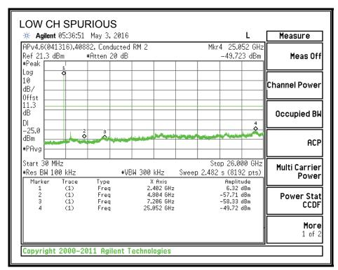
Note – Limit line should be -13.4 dBm for the Low Channel Spurious plot.
