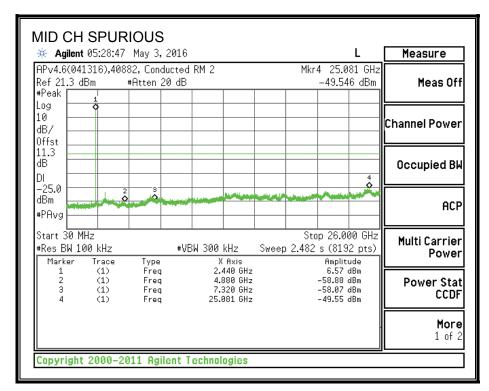
Note - Limit line should be -13.4 dBm for the Mid Channel Spurious plot.
