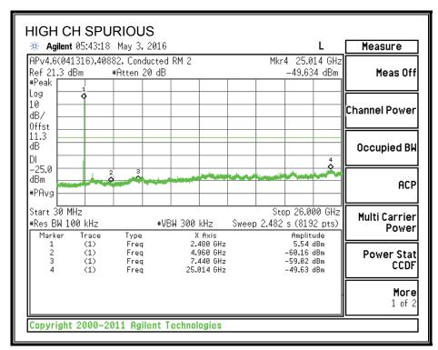
Note – Limit line should be -13.4 dBm for the High Channel Spurious plot.
