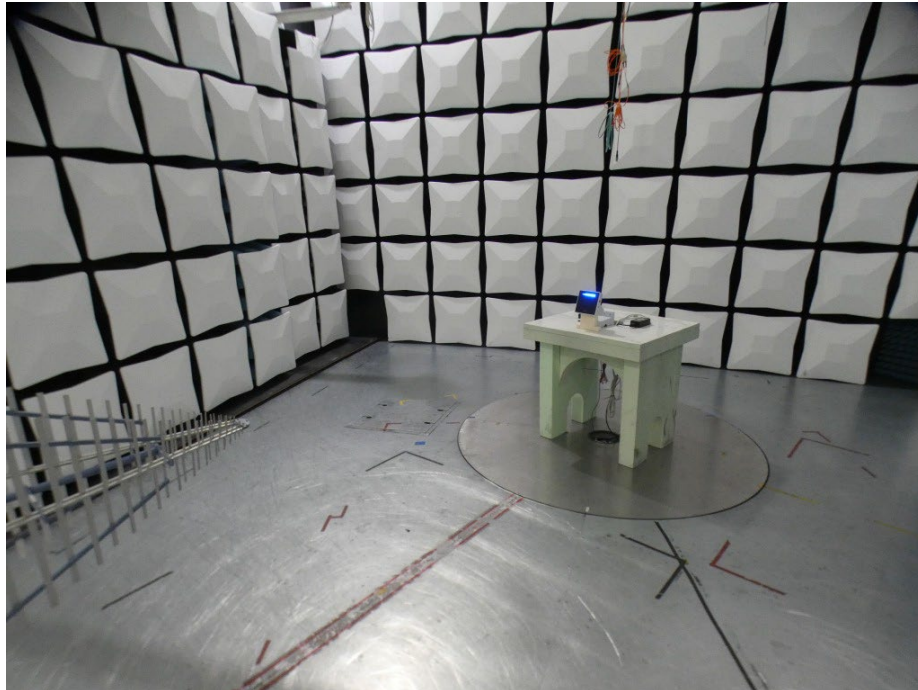
Photo 5: Test setup S01_AA01 for radiated emissions measurements up to 1 GHz in the semi anechoic room (SAR)
