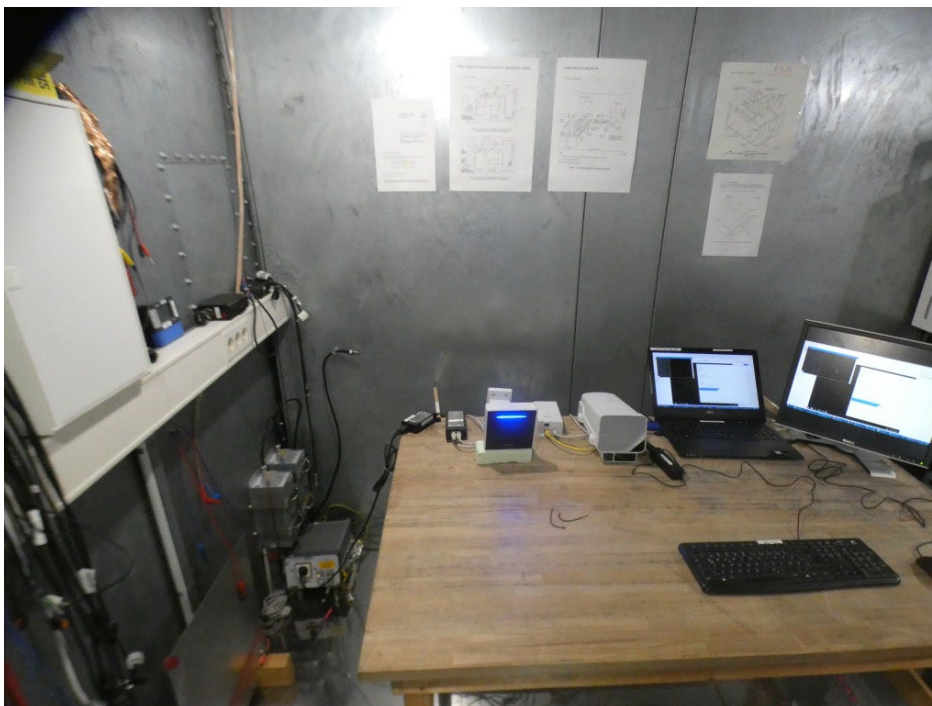
Photo 3: Test setup S01_AB01 for conducted emissions measurements below 30 MHz
