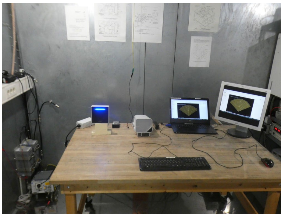
Photo 4: Test setup S02_AB01 for conducted emissions measurements below 30 MHz
