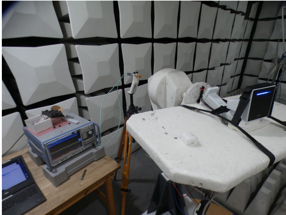
Photo 7: Test setup S01_AA01, for radiated emissions measurements above 26 GHz in the fully anechoic room (FAR)
