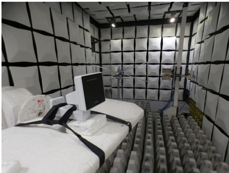
Photo 6: Test setup S01_AA01 for radiated emissions measurements above 1 GHz up to 26 GHz in the fully anechoic room (FAR)
