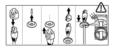
11. Pull the network cable back slightly so that the cable gasket adjusts itself on the cable.
