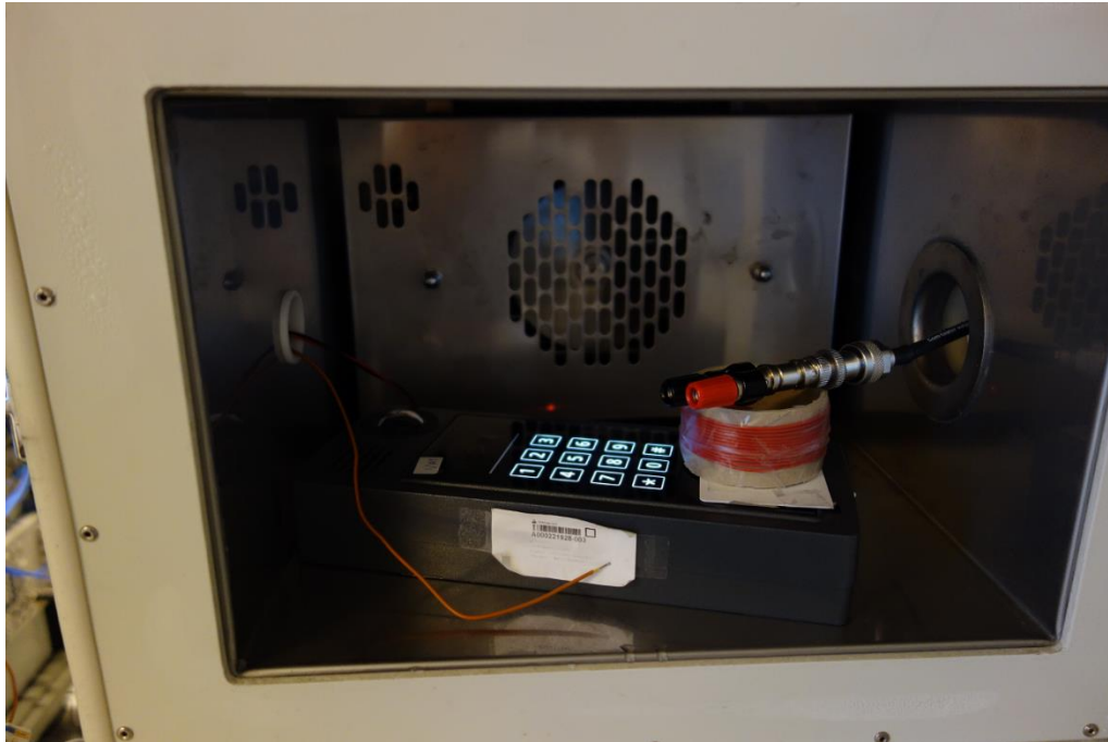
Photo of EUT in Climate chamber
