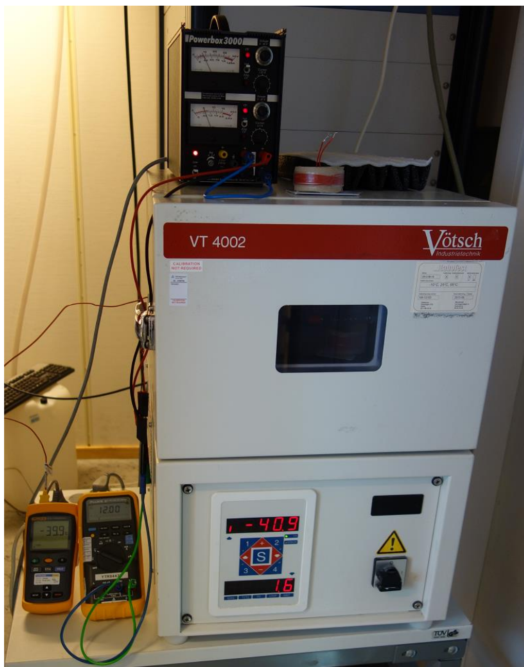
Photo of test setup with climate chamber
