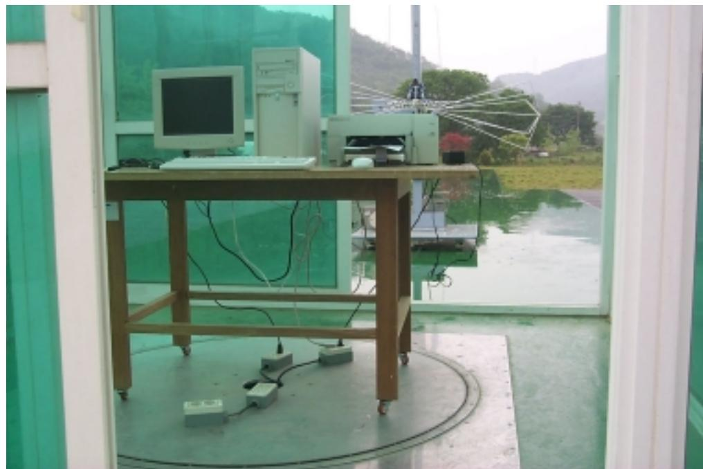
● Radiated Test Picture(Rear)
