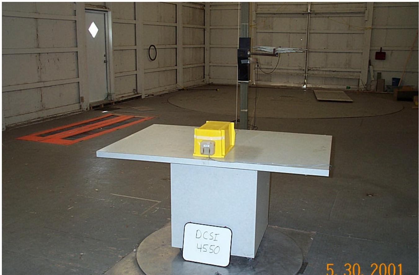
Since the EUT is wall mounted, it was placed in an upright configuration during the tests mounted on a nonconductive stand.
