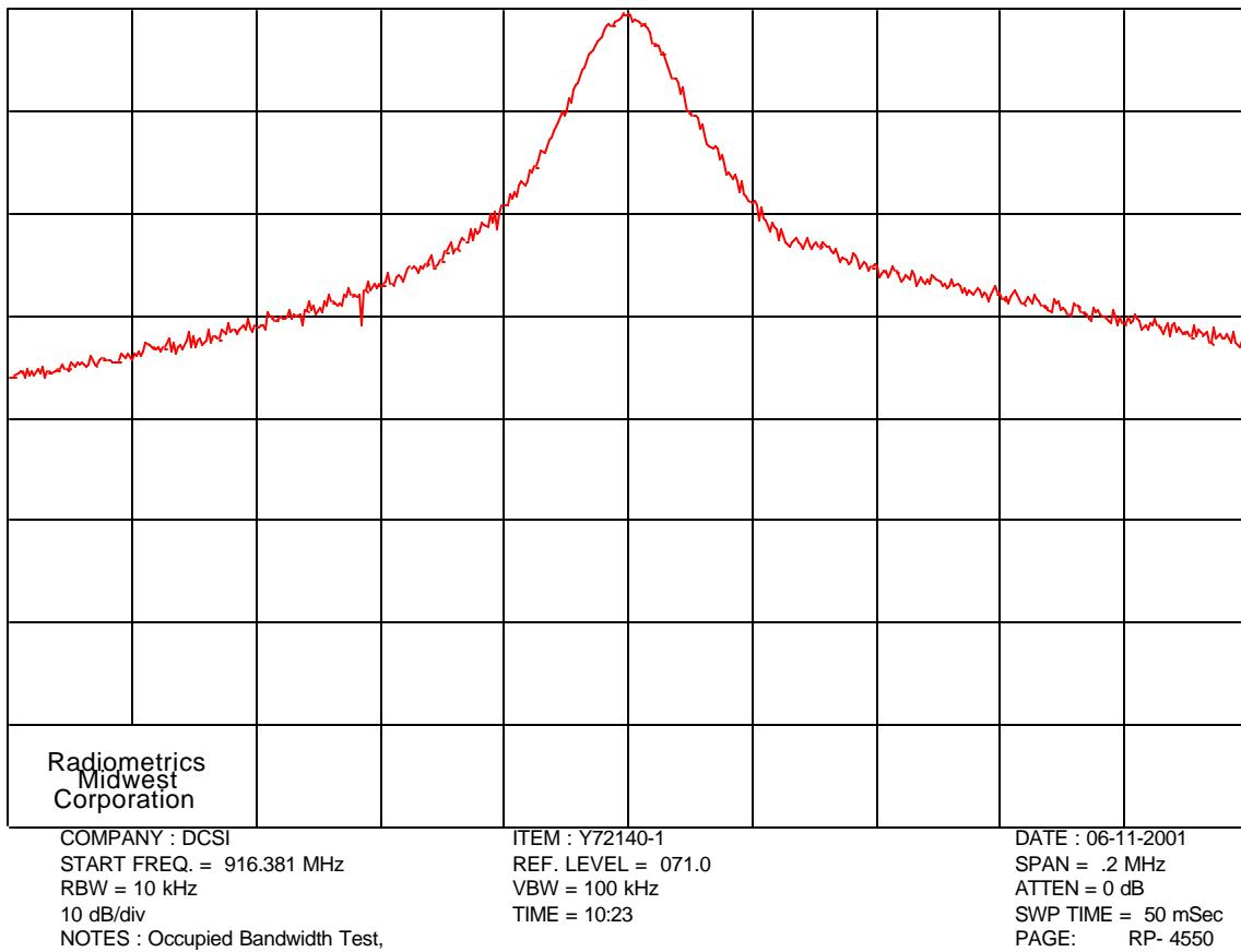
Test Result: 20 dB Bandwidth is 48 kHz.
