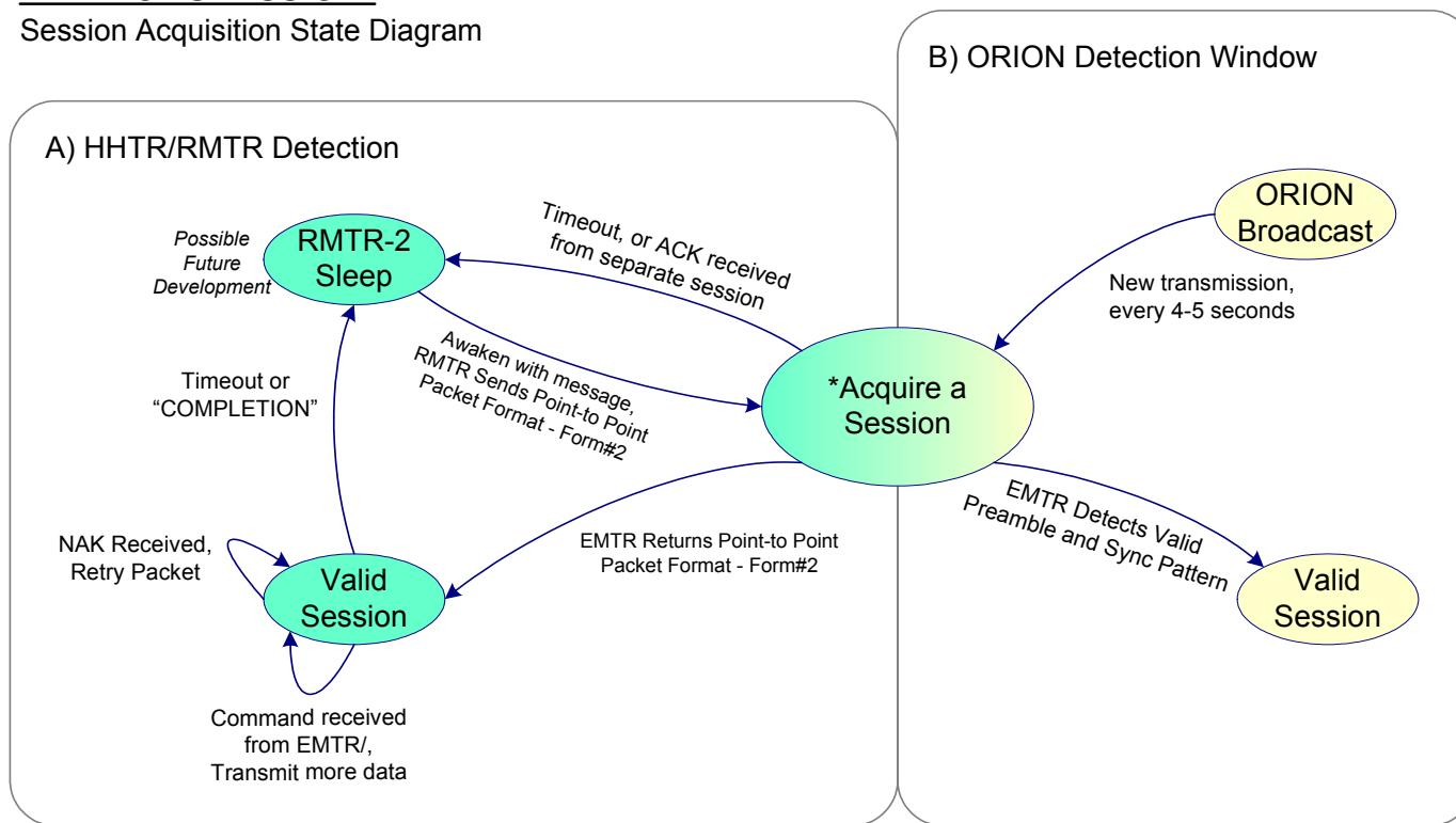
\*The EMTR constantly scans for incoming messages while time-slicing between two separate device protocols (See Y56111PDS Rev. -, section: 3.1.4). The following defines the processes within the "Acquire a Session" state above, for the two protocols:
