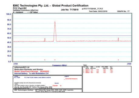
Channel 2480 MHz, Top Band Edge: Hopping off, Mark1 and Mark2 being set to around 2390MHz and 2483.5MHz
