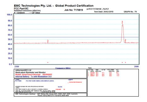
Hopping on, Mark1 and Mark2 being set to around 2390MHz and 2483.5MHz
