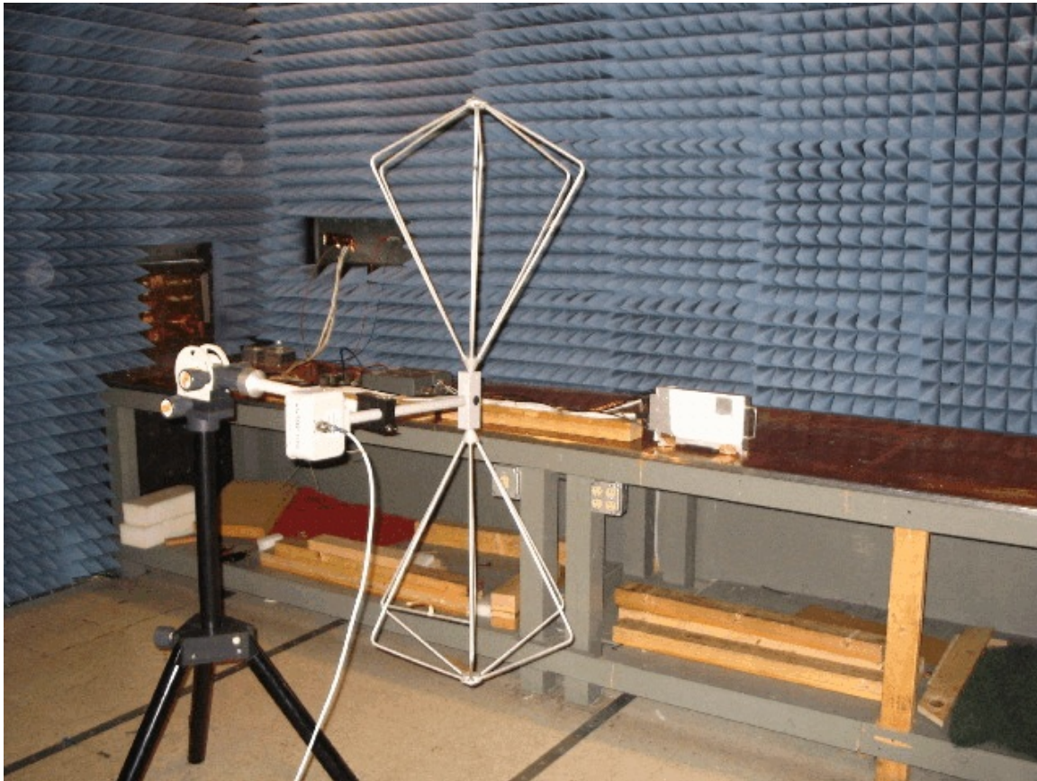
Figure 10-7 Photograph of Radiated Emissions Test setup Biconical Antenna, Vertical Polarization 30 MHz to 200 MHz
