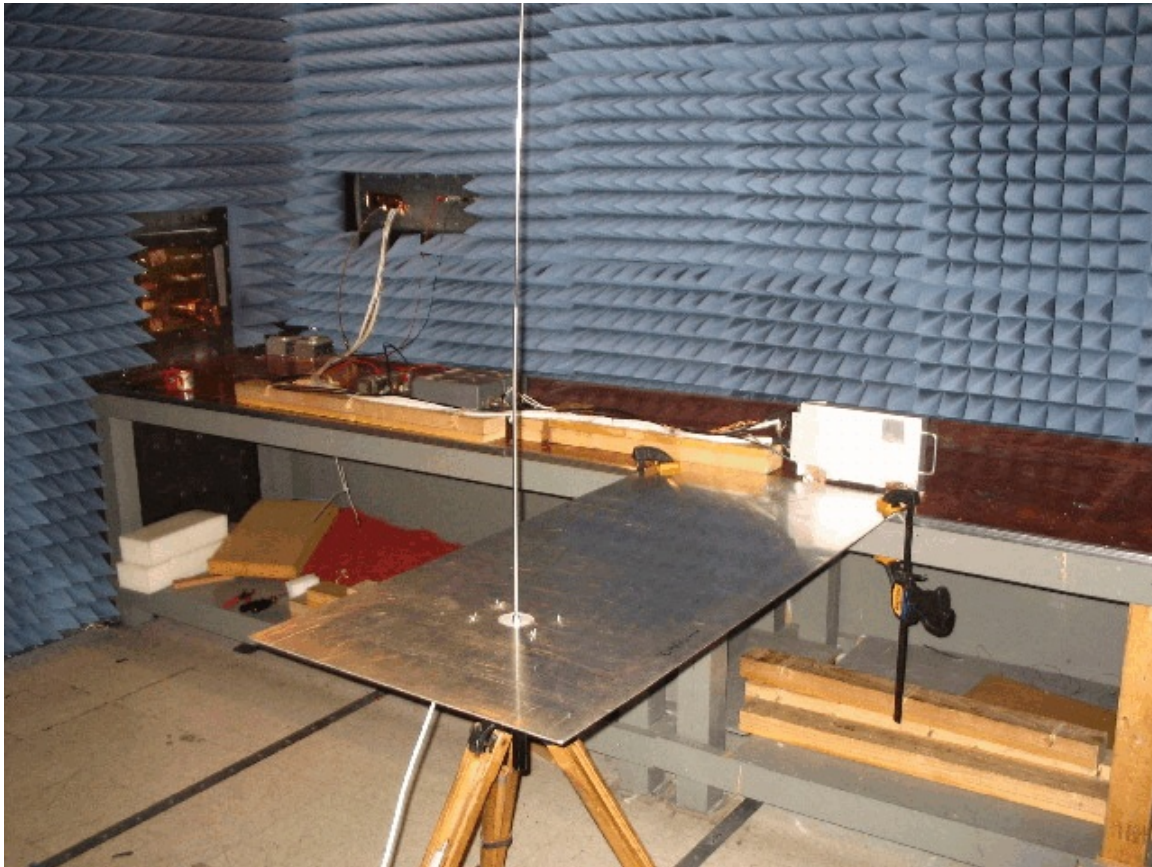
Figure I0-6 Photograph of Radiated Emissions Test Setup Active Rod Antenna 150 kHz to 30 MHz
