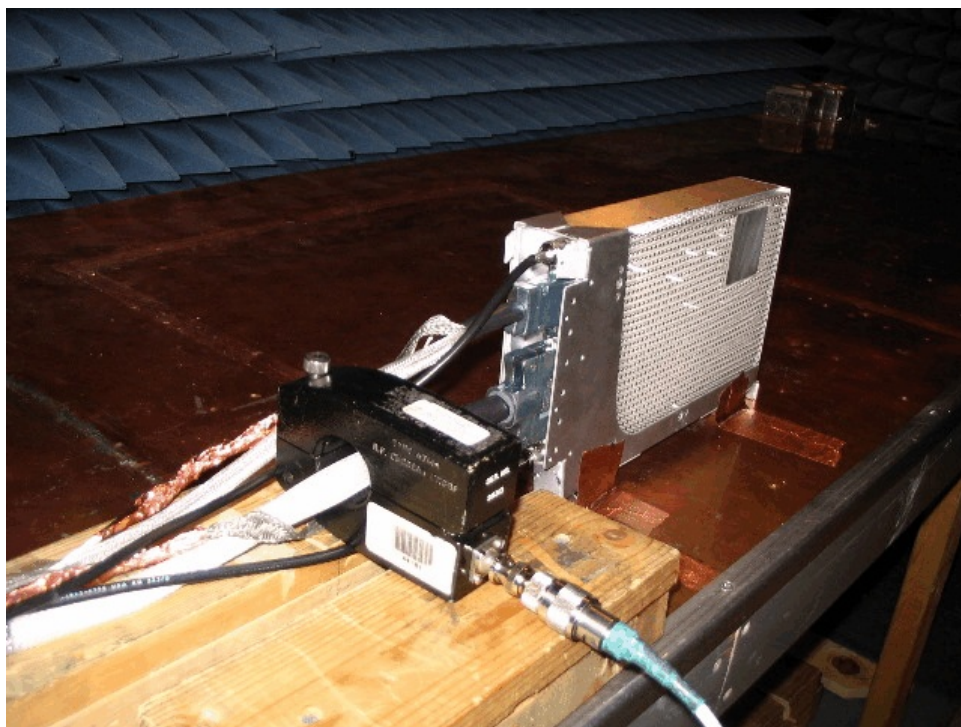
Figure 9-6 Photograph of Conducted Emissions Test Setup
