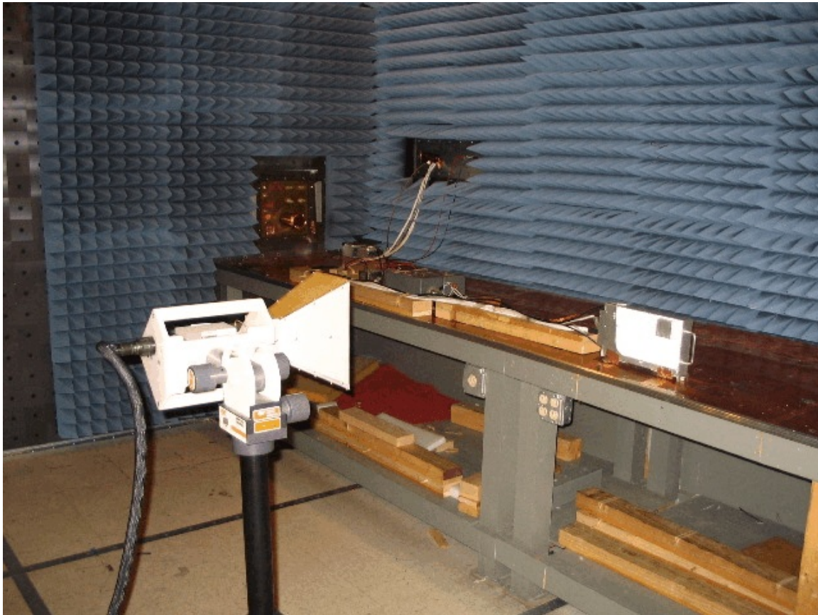
Figure 10-12 Photograph of Radiated Emissions Test Setup Horn Antenna, Horizontal Polarization 1 GHz to 6 GHz
