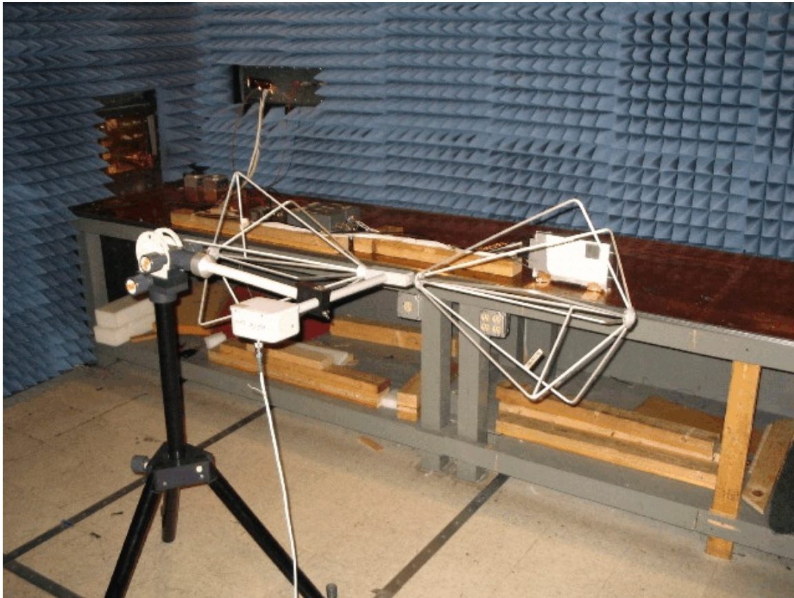
Figure I0-8 Photograph of Radiated Emissions Test Setup Biconical Antenna, Horizontal Polarization 30 MHz to 200 MHz
