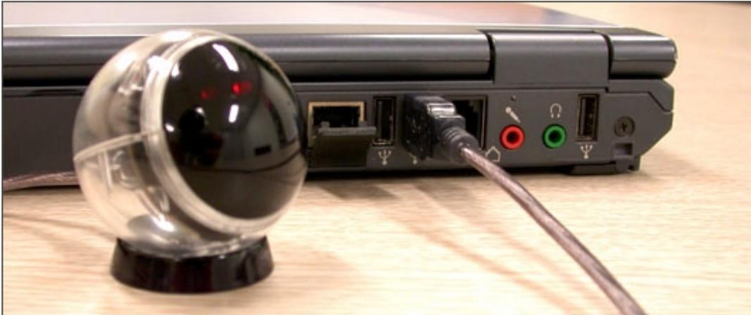
Once the iMON Station is connected to the USB port, Windows detects your iMON Station automatically and performs required process. **Please see the installation guide for the OS installed on your PC.**
