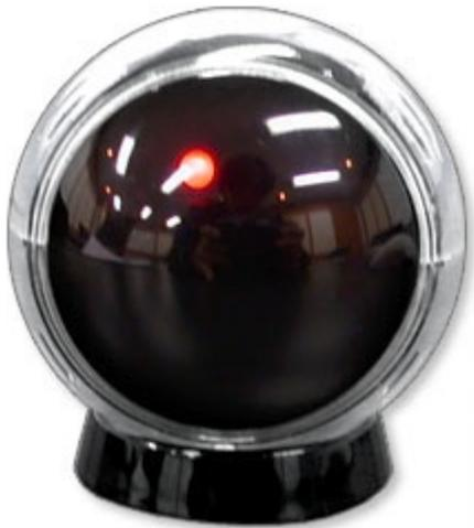
Analyze the IR signal received from the remote controller and **deliver the result to PC**. Use the **enclosed mount** and **dual-faced tape** to install this product on the **inclined surface**. When you use the mount, you can use the hole at the bottom of the product to **adjust the signal reception angle**.
