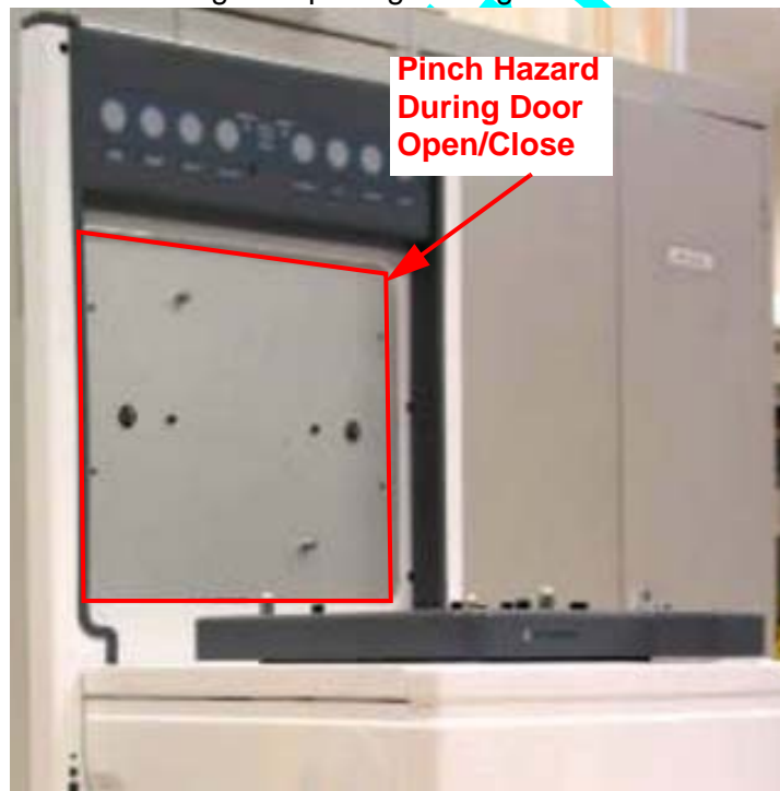
FIGURE 2 Pinch Hazards During Service
